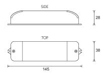
The Relco 30W Driver is suitable for use with our constant current Domino Surface and Recessed luminaires. It is for use with the luminaires wired in series. The driver has thermal protection, short circuit protection and screw down cable clamps. This power supply is dimmable with a 1-10V control signal.
