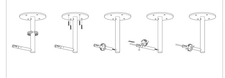
**NOTE** when installing Horizontal Standoff, be sure to align the pillar with the system before drilling holes to ensure the bracket will line up correctly when installed.
